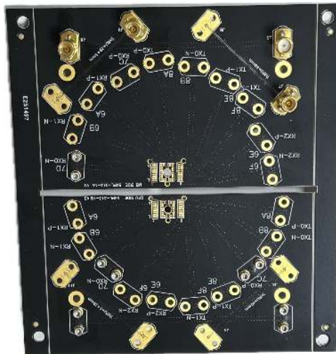
5R01T01 U3 open,short,Load calibration 5R01T02 U3 1X,2X calibration fixture 5R01T03 U3 TRL calibration fixture 5R09T01 U3 Female fixture
